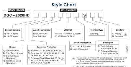
Use of the 87G and 87N elements, generator protection selection D, requires enhanced sensing, bus inputs selection E.
